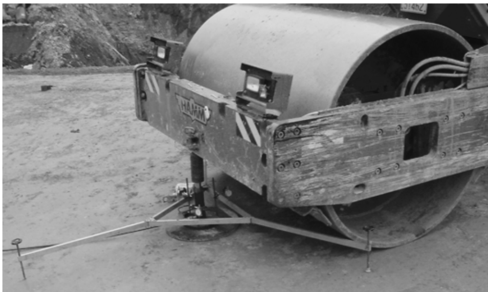
Fig 3. The Plate Bearing Test
